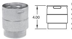
Use as a connector between stove exhaust collar and the positive twist lock of biomass chimney pipe. Order BSA when O.D. of exhaust collar is a true 3" or 4" dimension. Order BSAU when collar is less than 3" or 4" diameter.
