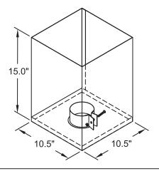
For use on open beamed pitched roofs or ceilings. Includes trim pieces for finishing out installation, also includes support band.
